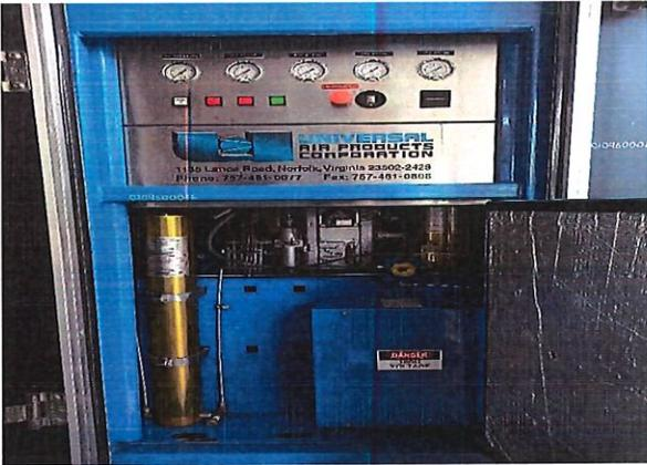
A close-up photograph of the air purification system. It features a control panel with several gauges and switches. Below the panel, there are two vertical cylindrical filters. The system is housed in a blue metal cabinet. Text on the panel includes "UNIVERSAL AIR PURIFICATION" and contact information for "1150 Limes Road, Norfolk, Virginia 23502-2428". | <p>Sistema de purificación del aire, marca MAKO</p>                           |
